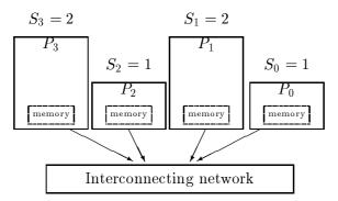
Figure 2: an *HBSP* with 4 processors
